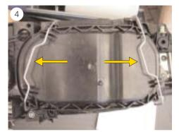
■ Push the headlight-cover fastening clamp outwards and remove this (see Fig. 4).
