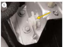
■ The headlight now has to be pulled forwards firmly in one go out of the additional guide.
