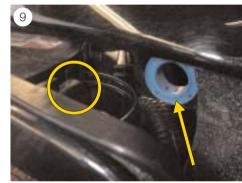
Refit all the removed parts in reverse order. When re-installing the headlight make sure that the guide on the headlight is inserted into to the holder (see Fig. 9, blue ring) first before the headlight is pushed completely into the bodywork. Check the lighting system to make sure it is in perfect working order. Check the headlight setting with the aid of diagnostic equipment if necessary (fault-code readout, basic setting of headlight range adjustment etc.).
