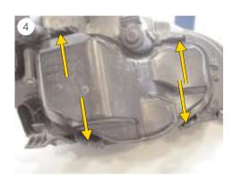
■ Press the locating lugs out of the mounting brackets on the headlight cover and remove this (see Fig. 4).
