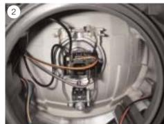
■ Loosen the spring-wire clamp and replace the H4 bulb (see Fig. 2).
