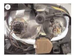
■ Press the locating lugs out of their holders on the headlight cover on the top and bottom of the headlight and remove them (see Fig. 4 and 5).
