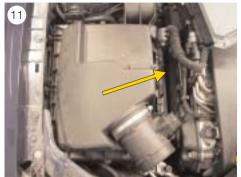
■ Pull the air filter box out of the guides (diagonally upwards to the right) (see Fig. 11). This pulls the hose out of the crankcase ventilation at the same time (see Fig. 12).
