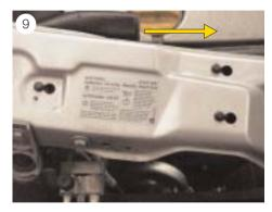
■ Pull the air intake channel to the right (see Fig. 9).)
