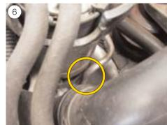
■ Bend the fuel filter carefully to one side. Note! Watch the refrigerant line in vehicles with air conditioner system (see Fig. 6).
