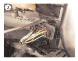
■ Separate the plug connection at the headlight. Use a screwdriver to loosen the catch and then pull the central plug off (see Fig. 3).
