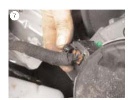
■ Loosen the plug connection and pull the plug off the headlight (see Fig. 7).
