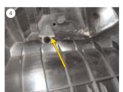
■ Pull the rubber bolt in the lower part of the air filter box upwards and out (see Fig. 4).
