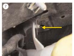
Loosen the fasteners of the filler neck (window cleaning system) (see Fig. 7).
