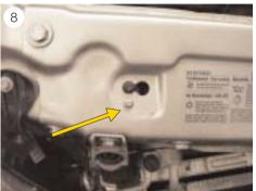
■ Unscrew the fastening screw (Torx 20) from the air intake channel (see Fig. 8).
