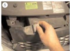
■ Loosen the screws from the plastic grille and remove this (see Fig. 5).
