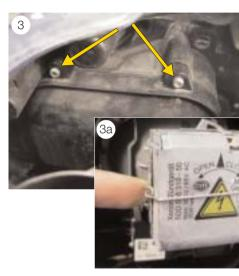
Then fold the cover back as far as possible and pull it upwards and out of the mounting brackets (see Fig. 3).
