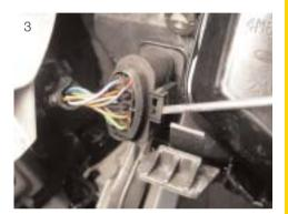
■ Separate the plug connection at the headlight. Use a screwdriver to loosen the catch and then pull the central plug off (see Fig. 3).
