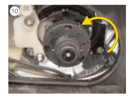
■ Remove the screw attachment of the xenon bulb and replace the bulb (see Fig. 10).
