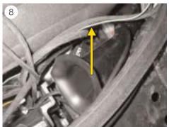
At the same time, pull the front part of the air intake channel forwards and take it out of the engine compartment (see Fig. 8)
