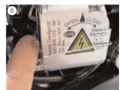
■ Loosen the fastening clamp on the headlight ignition module (see Fig. 6).
