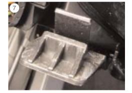
Refit all the removed parts in reverse order. When inserting the headlight make sure that the lower two mounting brackets of the headlight (see Fig. 7) are properly locked in place on the body.
