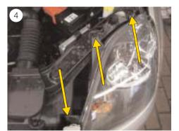
■ Unscrew the fastening screws (Torx 30) from the headlight (see Fig. 4).
