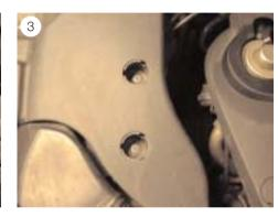
■ Remove the cover caps from the fastening screws, remove the screws (see Fig. 3) and take the plastic cover off.
