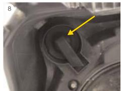
■ Pull the rubber cap off the parklight, remove the socket with bulb from the reflector and replace the bulb (see Fig. 8).
