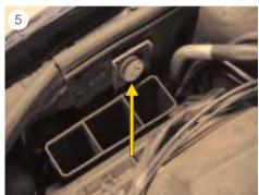
■ Remove the fastening screw from the air filter box (see Fig. 5).
