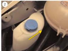
■ Pull the water tank off the threaded bolt and push it towards the rear (see Fig. 2).
