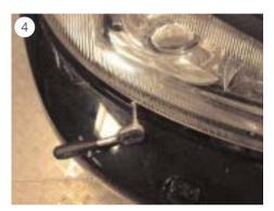
The lower fastening screw is located between the headlight and the front apron see Fig. 4).
