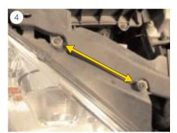
■ Remove the fastening screws (see Fig. 4).
