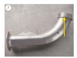
■ The air intake channel comprises two parts and can be separated.
