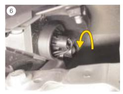
■ Turn the bulb socket to the left and then remove it from the headlight with the bulb (see Fig. 6).
