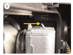
■ Press the fastening clamp for the supply cable towards the rear (see Fig. 6).
