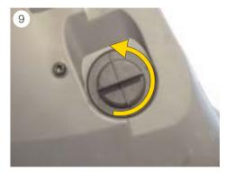
■ Turn the indicator socket base to the left as far as it will go and remove it from the headlight together with the bulb. Replace the bulb (see Fig. 9).
