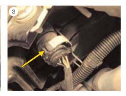
■ Push the lock on the connecting plug sideways (see Fig. 3) and then remove the plug from the headlight.
