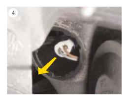
■ Pull the plug-in base backwards out of the reflector and replace the bulb (see Fig. 4).
