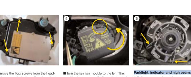
■ Remove the Torx screws from the headlight cover and take this off the headlight (see Fig. 4).
