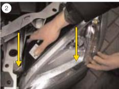
■ Reach behind the headlight with one hand. Then pull the headlight forwards firmly in one go and remove it from the bodywork (see Fig. 2).
