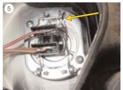
■ Loosen the spring-wire clamp and replace the bulb. (see Fig. 5).
