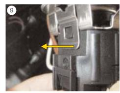
■ Use a screwdriver to push the fastening clamp outwards so that it fits over the locating lug (see Fig. 9).
