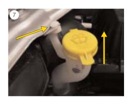
■ Remove the filler neck of the washer fluid
