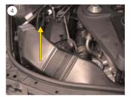
■ Pull the air channel upwards and off the air filter box (see Fig. 4).
