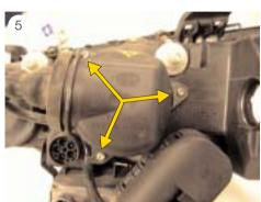
■ Unscrew the screws on the cover cap (see Fig. 5) and remove the cap.
