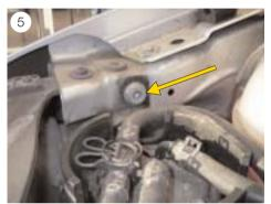
■ Grasp the parklight-bulb socket by the connecting plug and pull it out of the reflector (see Fig. 4).
