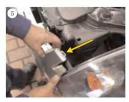
■ Pull the front trim forwards slightly and remove the headlight from the bodywork (see Fig. 6).
