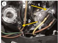
■ Loosen the spring-wire clamp and replace the bulb (see Fig. 5, no. 1).
