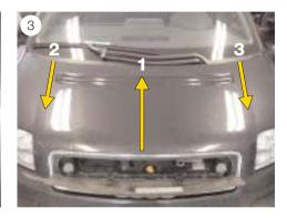
■ Lift the bonnet at the front (1), then pull it forwards and out of the rear guides (2) and take it off completely (see Fig. 3).
