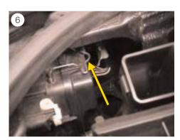
■ Replace the bulb in the same way as on the passenger side (see Fig. 6).
